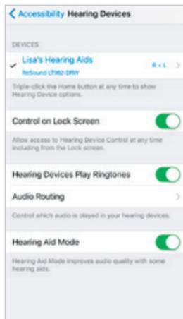
Audio Routing allows you to control how different audio inputs will be directed.
